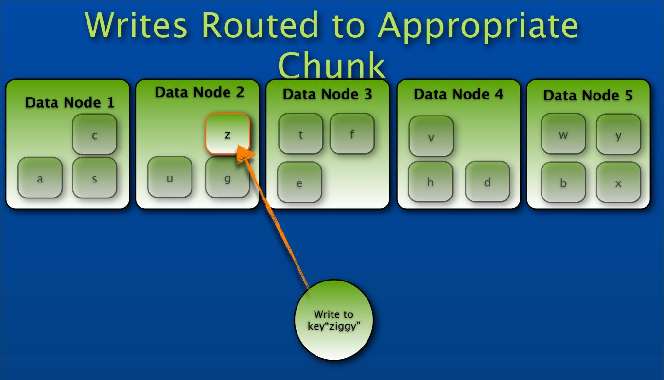
Writes are efficiently routed to the appropriate node & chunk
