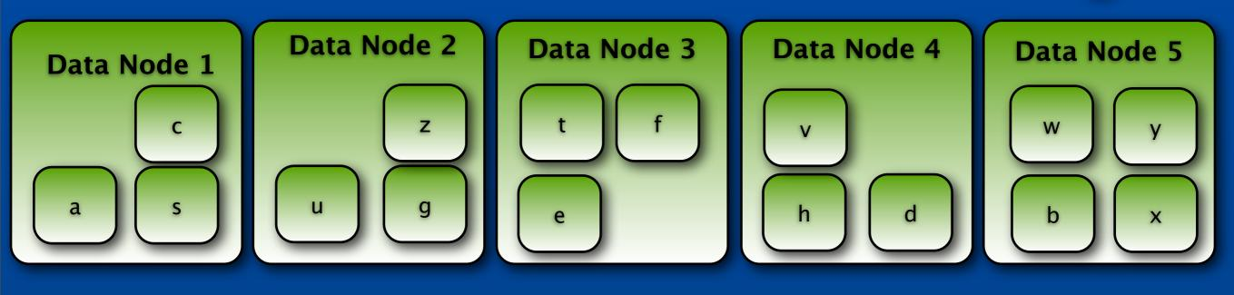
The goal is equilibrium – an equal distribution. As nodes are added (or even removed) chunks can be redistributed for balance.
